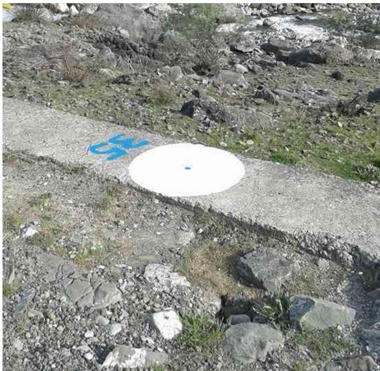
Figure 6: Ground mark with 1m diameter painted in white to be visible in an aerial image (source: Hansa Luftbild AG, 2016)
